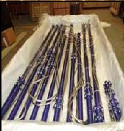
Level alarm, temperature & water bottom measurement systems 01817.
